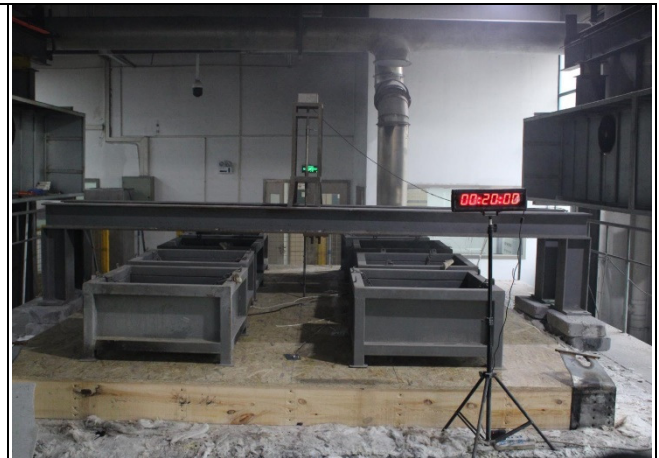
Photo 18: The unexposed face of sample (After test duration of 20 minutes)
