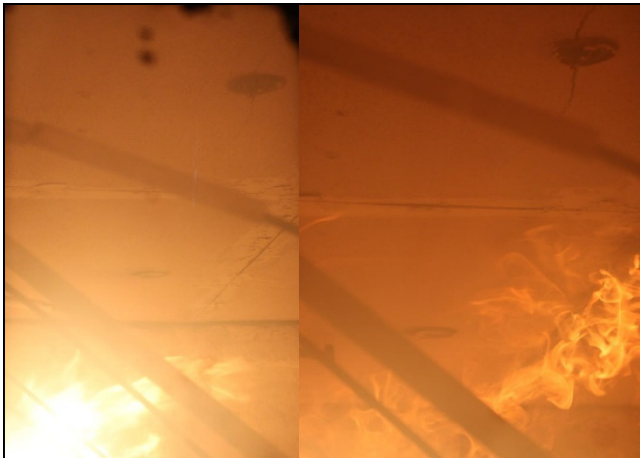
Photo 17: The exposed face of sample (After test duration of 10 & 15 minutes)
