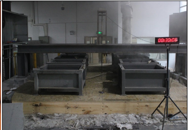
Photo 20: The unexposed face of sample (After test duration of 30 minutes)
