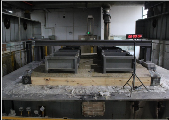
Photo 15: The unexposed face before the test (Distribution of the weights)
