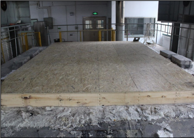
Photo 13: The unexposed face before the test
